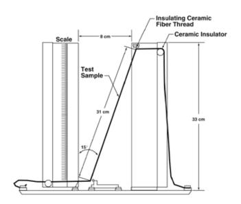
Figure 2. Sketch of apparatus fo NASA NHB 8060.1C, Test 4, Electrical Wire Flammability Test.
