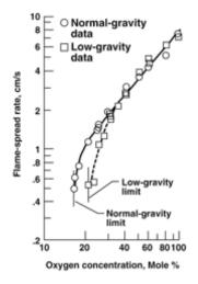
Figure 4. Experimental data on flame-spread rates and flammability limits of thin-paper fuels for downward normal gravity and quiescent microgravity [39].
