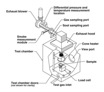
Figure 3. Sketch of apparatus for NASA NHB 8060.1C, Test 2, Heat and Visible Smoke-Release Rates.
